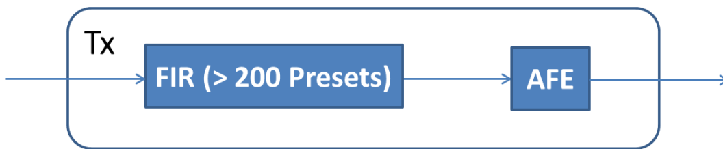
Figure 6: Typical Tx Device Blocks
