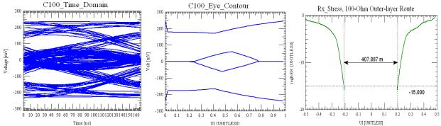
Figure 14: HDD Rx Compliance Plots, 100-Ohm Route
