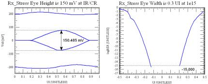
Figure 11: Performance of Rx Compliance Stress Circuit as Measured by CA
