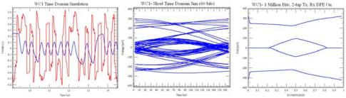
Figure 26: WC1 Channel Initial Simulations
