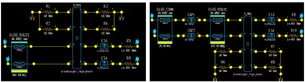
Figure 17: HDD Implementation Configured for S-Parameter Measurement
