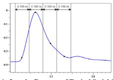
Figure 6: Impulse Response of Typical Serial Channel
