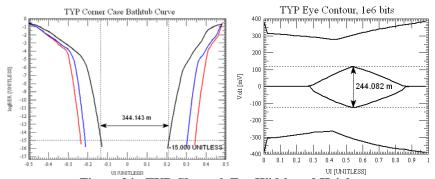
Figure 24: TYP Channel, Eye Width and Height
