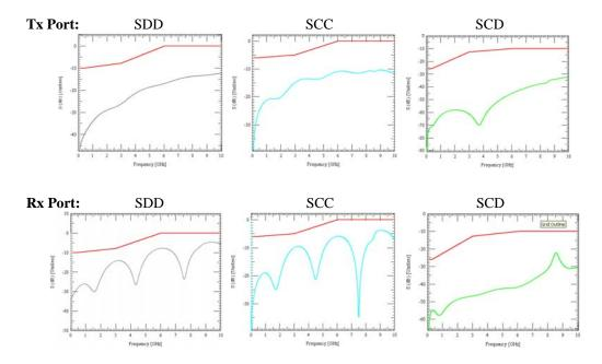
Figure 18: Compliance of HDD Passive Interconnect S-Parameters to SAS Limits
