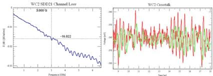
Figure 34: WC2 Channel Loss and Crosstalk
