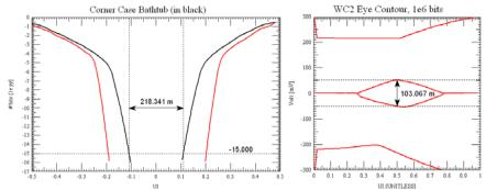
Figure 37: WC2 Channel Eye Width and Height
