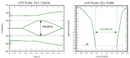
Figure 8: CA Results from Tx Compliance Simulation
