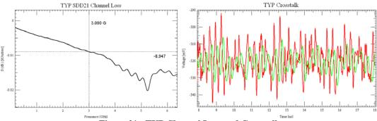
Figure 21: TYP Channel Loss and Crosstalk
