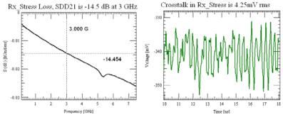
Figure 12: Loss and Crosstalk Performance of Rx Compliance Stress Circuit
