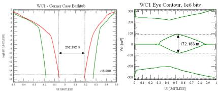
Figure 31: WC1 Channel Eye Width and Height
