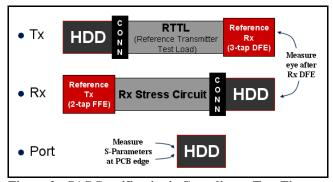
Figure 2: SAS Specification's Compliance Test Fixtures
