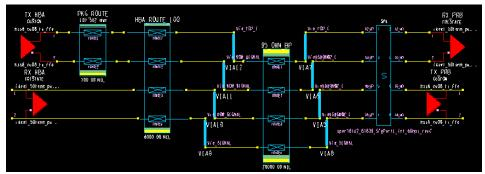
Figure 10: Testbench Circuit for Rx Compliance Stress Testing
