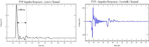
Figure 22: TYP Channel Impulse Response
