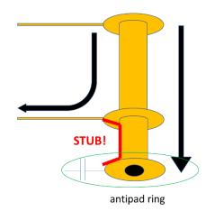
Figure 14: Stub lengths include pads, if not removed
