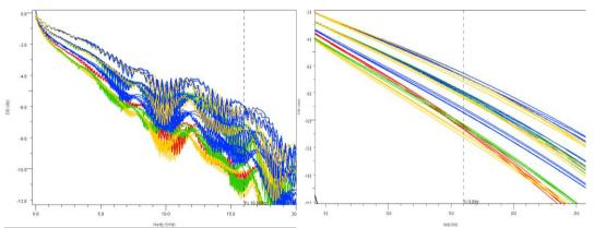
Figure 6: MCIO Cable Measured IL, raw (left) and linearized (right)
