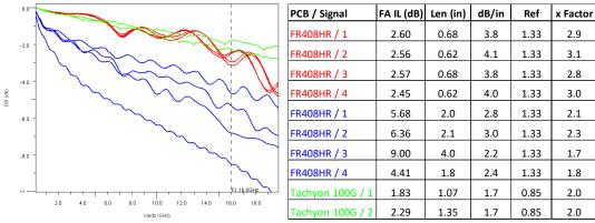
Figure 4: Measured Microstrip IL Across Three PCBs
