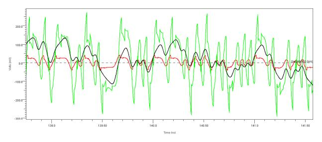
Figure 20: Rx input (black) applied to spec EQ (red) and Xconn IC (green)
