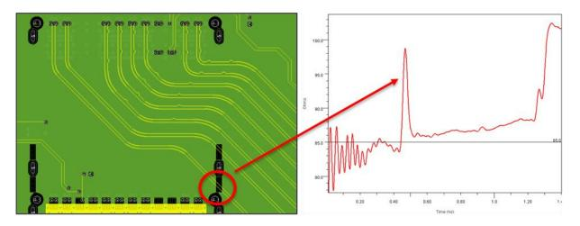
Figure 17: Unexpected Discontinuity due to Plane Cutout
