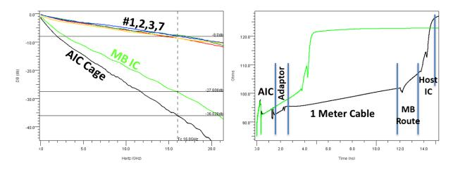
Figure 3: Simulations of Gen5 Loss Budget Scenarios
