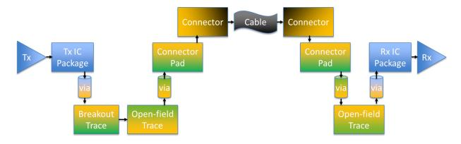
Figure 10: Typical set of discontinuities in a Gen5 Tx to Rx path
