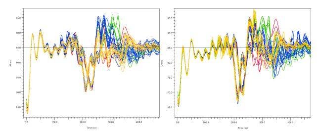
Figure 15: Cable connector impedance measurements, four vendors (by color)
