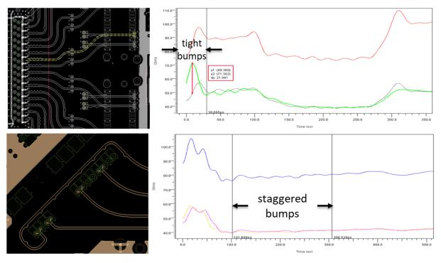
Figure 13: Correct (lower) and incorrect (upper) p/n length matching
