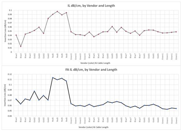
Figure 7: MCIO Cable Loss, 36 Measurements
