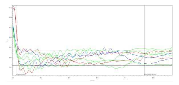
Figure 12: Differential impedance range and variation of breakout traces
