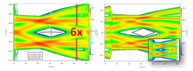
Figure 21: Eye diagrams, Xconn IC (left) and Reference (right) EQ
