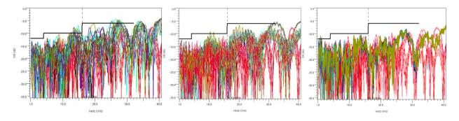
Figure 18: Using IL to damp reflections and meet RL mask
